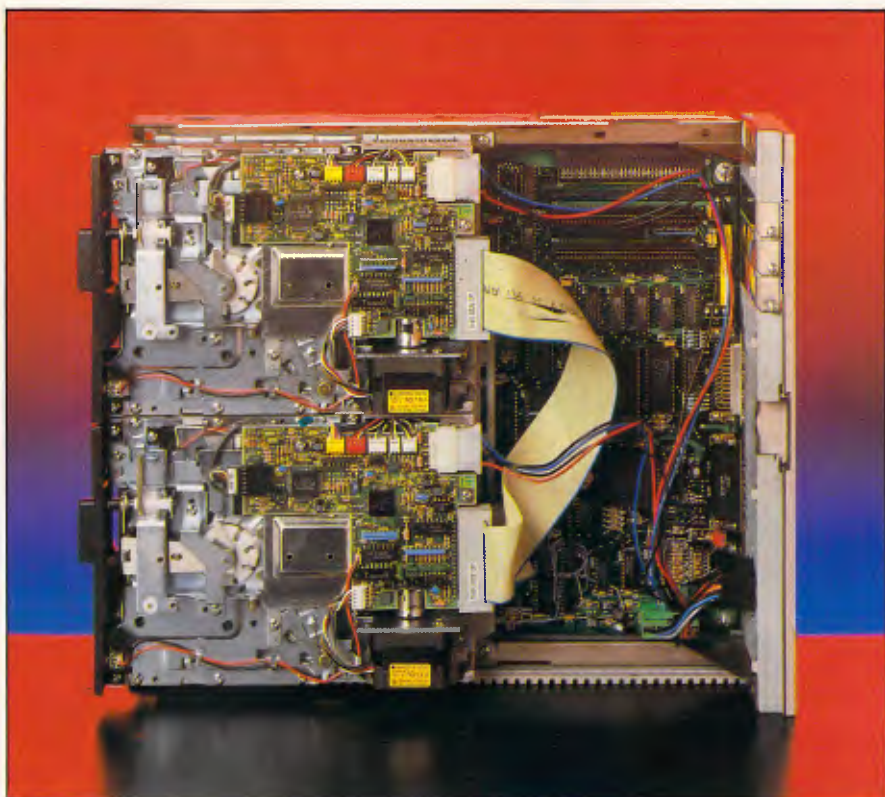
The main PCB is well built and occupies the entire base of the unit
